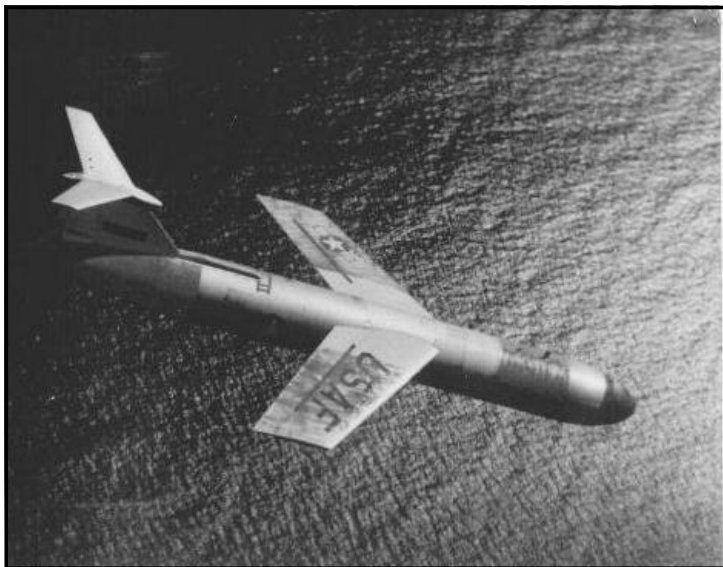
CGM-13A Mace Serial Number 58-2467 Shown here going into the Ocean at the end of it's flight Speed App. 525 Alt. 3,000 Ft.
