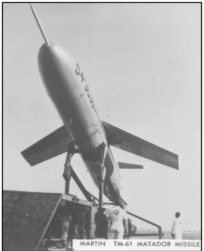
Member James Bass , Newport, KY sent in this photo of a bird in its morphing phase between being a Matador B and Mace A. The photo is labeled Martin TM-61 Matador Missile but as can be seen it has the distinctive profile of the later Mace A.
